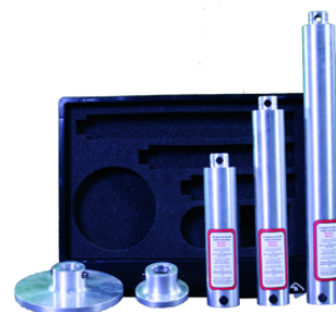
Accessory case: ram extensions and cross ramming heads
