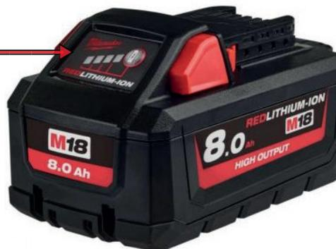
If the battery is not used for a long time, the battery will switch to standby. To be able to use it again, the battery must be reactivated (charged). The charge status can be accessed by pressing the button on the battery (see fig.). The battery can then remain in the equipment (the equipment must however previously be off for at least 1 minute) (if not the display is imprecise). The number of LEDs lit corresponds to the state of charge.
