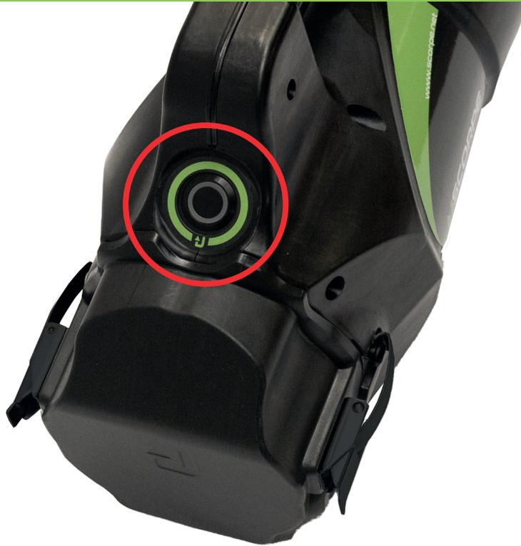
To start the battery powered equipment, press the on / off switch (1). The switch turns green. The battery powered equipment is controlled by the handle lever / control handle. The speed of movement is adjusted by pressing more or less. The maximum cutting or spreading force / pressure requires a full operation of the handle lever.
