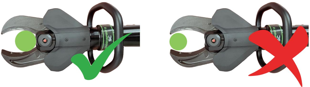
To prevent damage to the blades, they must always be positioned at right angles to the work piece. In addition, the shear blades must not be more than 5 mm apart from each other at the tips during the cutting cycle. If this value is exceeded, the cutting cycle must be interrupted and the blade must be repositioned.
