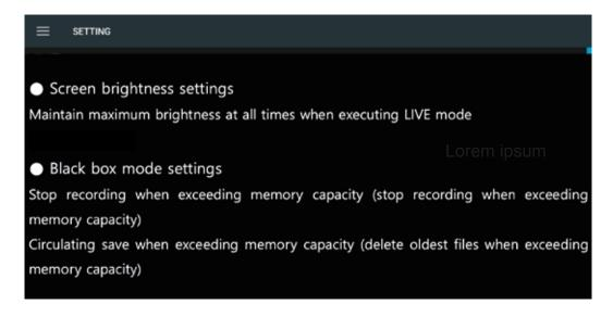
**Screen brightness settings** - Screen brightness can be adjusted manually. It can be set to maintain maximum screen brightness when executing LIVE screen.
