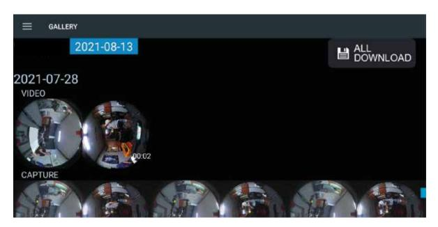
The BVA7 camera saves videos and photos in the internal memory of the camera. Saved data can be saved and moved to tablets or mobile devices, and it can also be selected for deletion.
