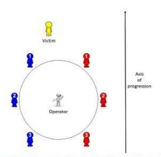
In this case, the sensors 1 blue and 1 red detect a signal. We will then use the point that captures the most important signal (1 blue) as the new center of the search circle as expressed below:
