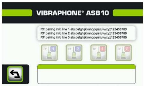
Press and hold the dimmed 1 blue icon. The icon will flash. Briefly press the sensor power-on button, which flashes rapidly. After 2 to 3 seconds the led stops flashing and becomes fixed. 1 blue icon on the control box is not dimmed no more.
