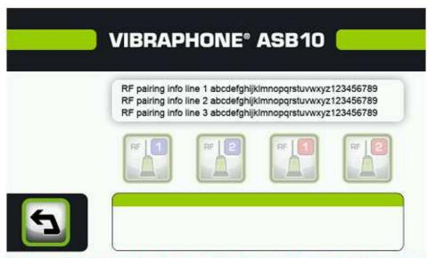
Be careful, you have to pair the sensors one by one. Make sure it is well charged. It is recommended to start with the 1 blue, 2 blue and so on. Here the 4 icons are grayed so the 4 sensors are not paired.
