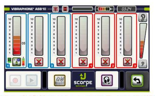
The icon on the left of the sensor icon changes state. The control unit and the sensor are connected together. The icon on the right of the sensor icon gives the charge level of the sensor.
