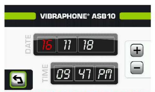
When holding an item it is displayed in red. After, one click on the other elements is enough. In red, the value can be changed by clicking on + or -. To change between morning and afternoon, clicking on AM or PM changes the value from one to the other.
