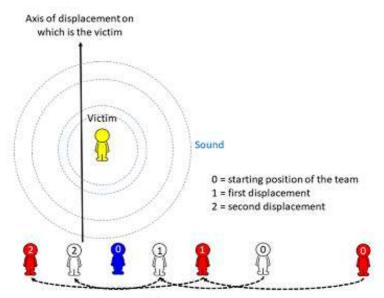
At the start the team is at position (0). The blue sensor has the strongest signal. The operator and the red sensor is getting closer to blue in half (1). The red sensor signal is still not as strong as blue. The victim is on the other side (2). The operator and the red sensor switches to the other side.
