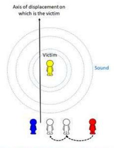
If at 2m from the blue sensor, the red sensor still does not perceive the sound as loud as the blue sensor is that the victim is on the other side of the blue sensor as follows:
