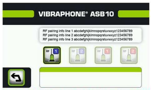
This screen indicates that the sensor of the 1 blue line is well paired with the control box. Proceed in the same way to pair the other sensors.
