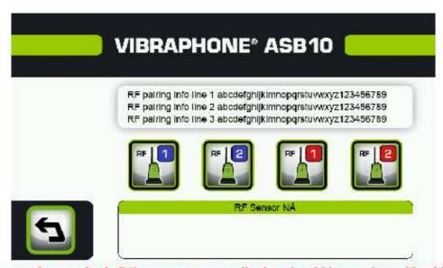
When you have paired all the sensors, your display should be as above (the 4 icons are no longer dimmed and the sensor leds are fixed).
