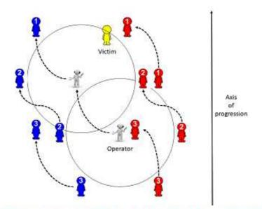
After this movement, the red sensor 1 will be the one that will capture the strongest signal. We then renew the operation of moving the operator according to the same principle. This gives us the situation below:
