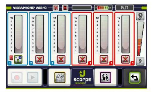
When the sensor is assigned to the line, it connects to the control box in wifi. The logo on the left of the sensor indicates that there is no signal. After a few seconds, the sensor status changes. It is displayed as follows:
