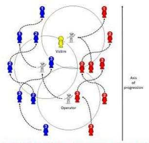
The displacement is repeated until the signal sensed by all the sensors is an equivalent intensity which means that the operator is over the victim.
