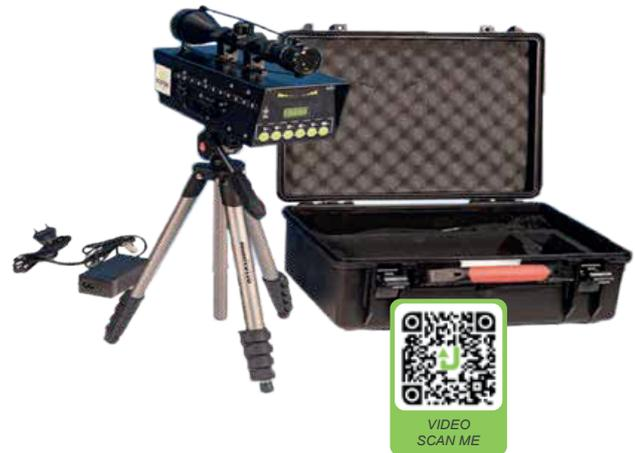
Developed in partnership with french USAR teams for their own safety during interventions. The range finder Scorp'Eye responds to movements from 0,20" to 0,40", measured on potentially hazardous masses such as floors, slabs, columns, walls, beams, trees ... It has also proved to be useful in the monitoring of industrial sites after a catastrophe.
